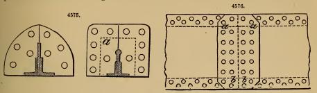
Inside Sheerstrakes .- The butts of inside sheerstrake should be double-riveted through inside sheerstrake and butt-strap; the row of rivets next butt of plate to be riveted fillesh before the outside sheerstrake is put on, Fig. 4576. aa, these two rows, through inside and outside sheerstrakes and butt-strap, and so on; bb, these two rows through inside sheerstrake, and butt-straps, and riveted flush, before outside plate is put on.
